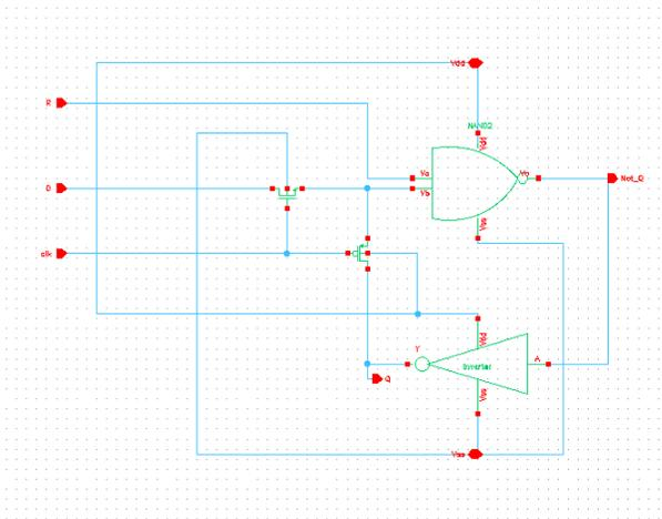
Figure 3 - Positive Level D-Latch with a Reset
