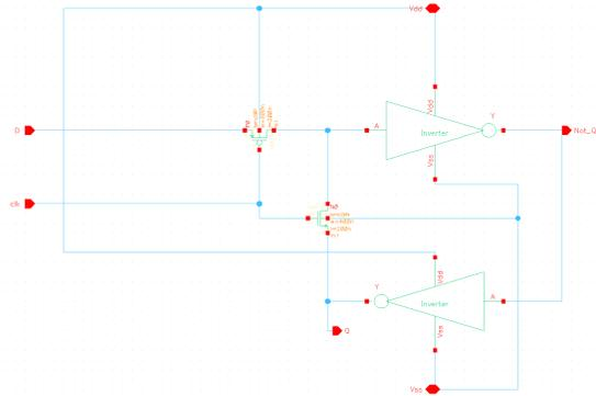
Figure 2 - Negative Level D-Latch
